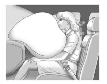
The outboard front passenger frontal airbag is in the instrument panel on the passenger side.
